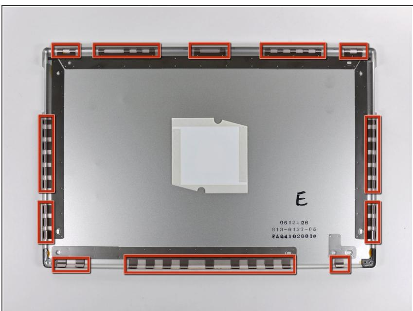
● The picture at left (rear panel already removed) shows the locations of the metal clips (shown in red) that snap on to the front display bezel. In the next few steps, you will use a small flathead screwdriver to release these clips from a ridge around the perimeter of the front display bezel.
